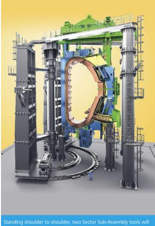
while carefully positioning and installing – via the rotary motion of the "wings" – the vacuum vessel thermal shields and two toroidal field coils. The sub-
